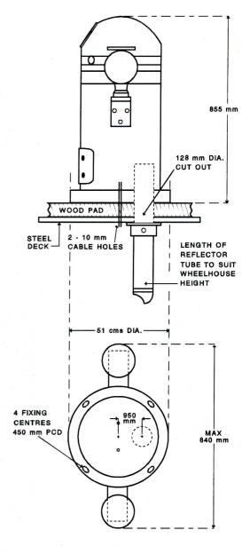
The York Binnacle can also be supplied without Deckhead Reflector Unit, for Steering or Standard Positions.
